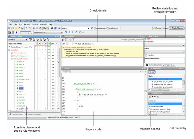
The Results Manager perspective has six sections below the toolbar. Each section provides a different view of the results. The following table describes these views.
